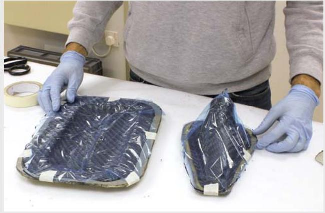
Tape the edges of the release film onto the back of the mould with some masking tape to hold it in place.
