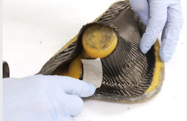
To create a perfectly straight seam at the back of the duct where the material meets, masking tape is used to mark a vertical line.
