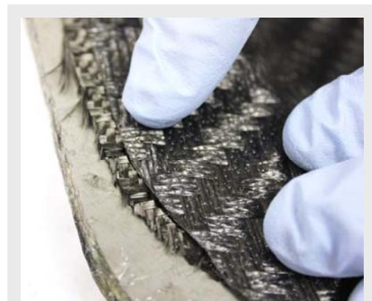
This close-up shows how later in the guide we will ensure that the backing ply/plies are slightly smaller than the surfacing ply, ensuring air paths to the surface are maintained.
