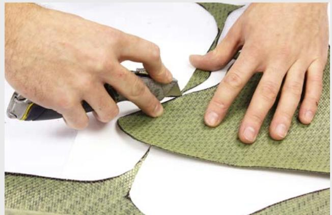
The backing ply is best cut using a Stanley knife on a cutting mat to avoid clogging shears.
