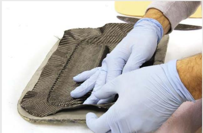
Continue to work the prepreg, gently smoothing and shaping it into the contours of the mould.
