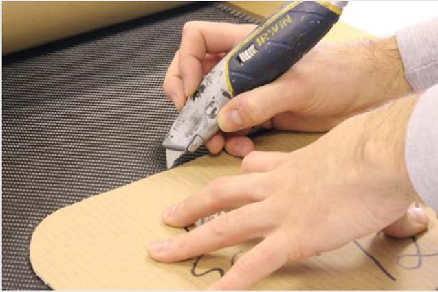
Instead of cutting, a Stanley knife blade is used at a right angle to 'score' the Easy-Preg to mark it.
