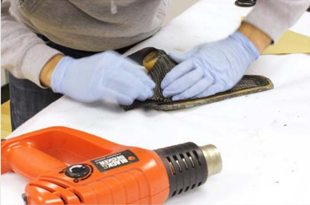
A very contoured shape like this NACA duct requires gentle application of heat to make the prepreg more pliable.
