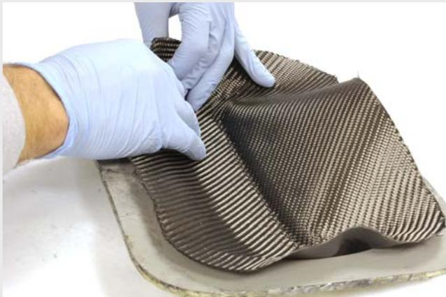
Start conforming the prepreg to the mould by pressing and smoothing it down on the flatter areas of the mould.
