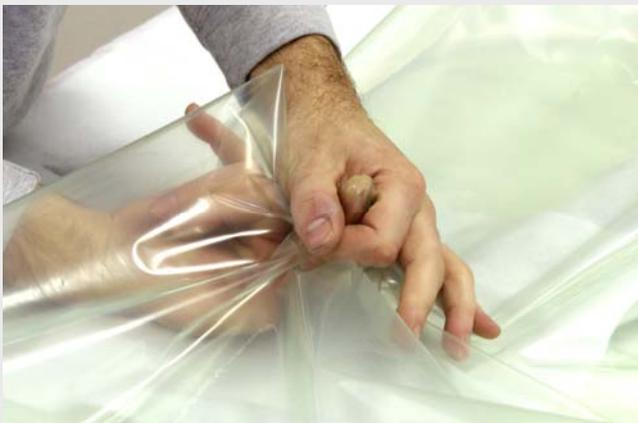
Make a 'peak' in the bagging film by pushing your index finger up from the inside of the bag.
