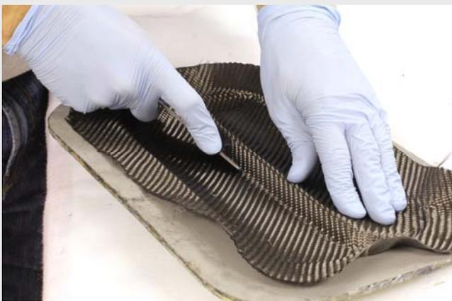
Use blunt tools (often home-made) to press the prepreg firmly into any tight corners or angles of the mould.
