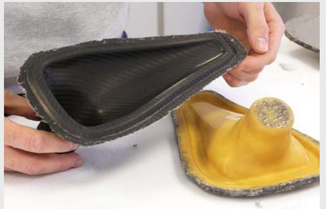
This NACA duct has a satin finish because the mould itself is satin finished.
