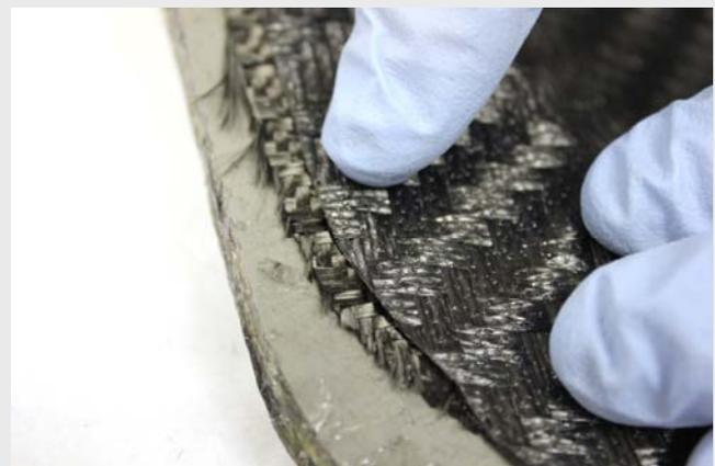
Having cut the backing ply smaller than the surface ply, a small amount of surface layer should extend past the backing layer all the way around the mould.
