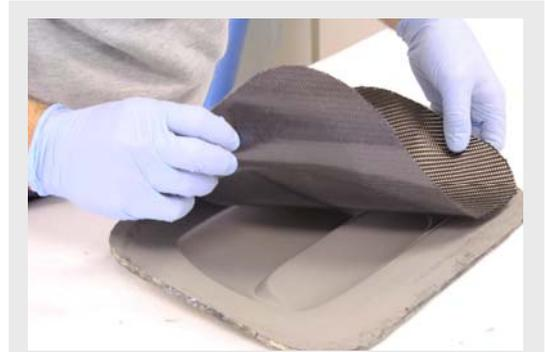
Easy Composites' Easy-Preg surfacing ply has a special solid resin film on one side only which is laid against the mould surface.
