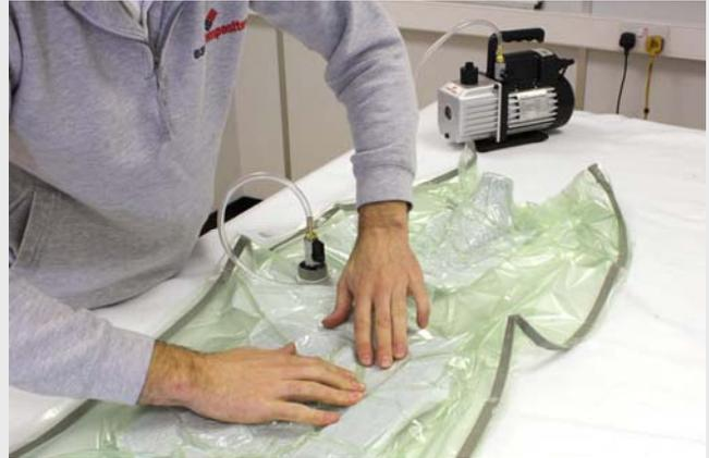
Push and pull the bag from side to side to free up more 'slack'. The whole surface should have an excess of bag.
