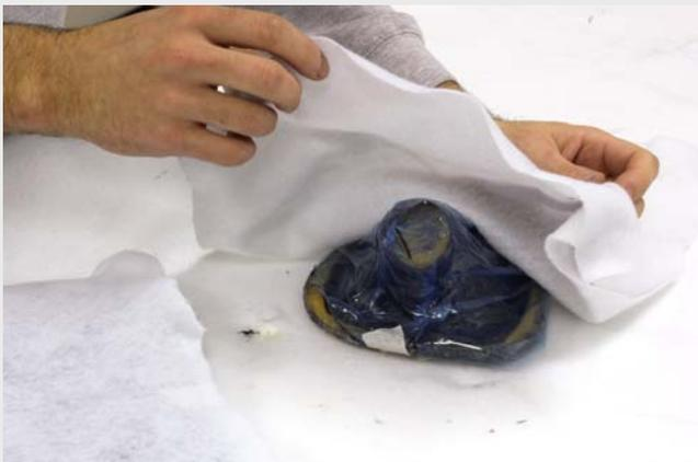
Roughly cut pieces of breather to cover your part(s). The breather cloth should be cut at least 60mm oversized so that it can loosely wrap the part.
