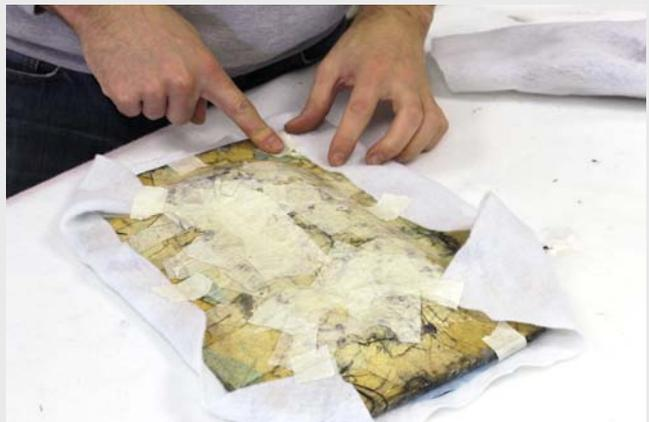
Use small pieces of masking tape to loosely hold the breather cloth in place by taping it to the back of the mould. This also prevents sharp edges on the mould from accidentally puncturing the bag.
