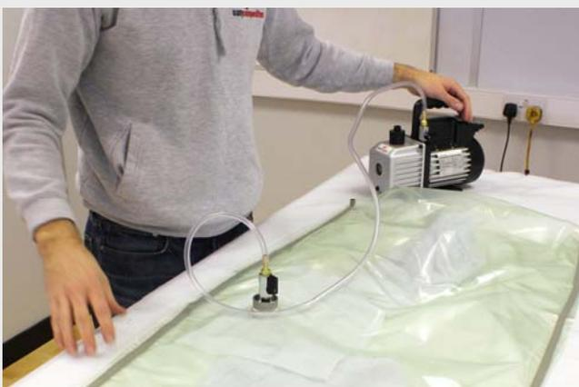
Connect the pump to the through bag connector using a length of silicone or PVC hose. Remember that silicone hose must be used on the part is in the oven.
