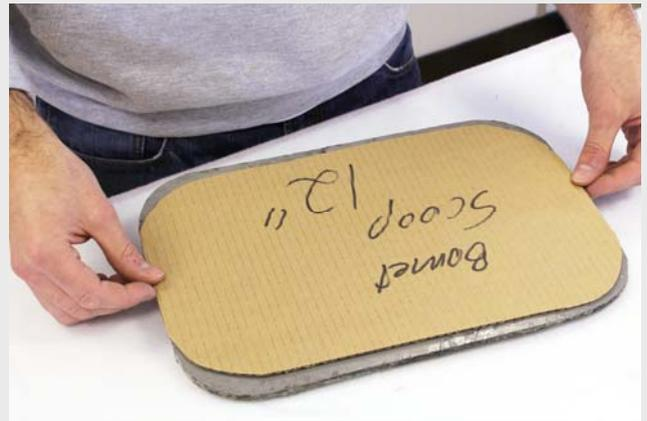
Simple shapes like the bonnet scoop can easily be templated using a piece of cardboard.
