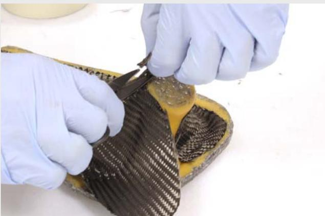
Composites Snips are useful for snipping off small excesses of material
