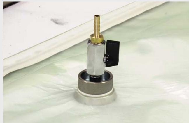
Screw the two halves together tightly to complete the through-bag connector fitment.
