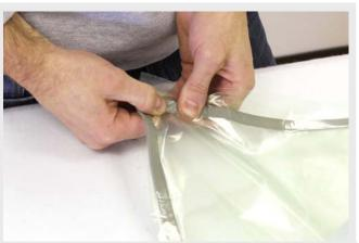
Always ensure you make the bag much larger than the parts. When using lay flat tube (LFT) bagging film, use the ready-made edges of the film where possible.
