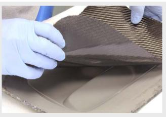
Gently lay the Easy-Preg down onto the mould, *film side down*.
