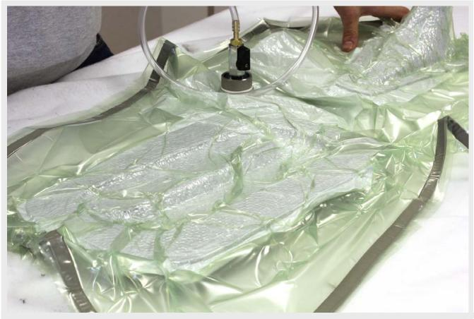
Correctly bagged parts under full vacuum. Plenty of wrinkles show there is an excess of bag on both parts.
