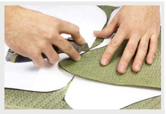
The backing ply is best cut using a Stanley knife on a cutting mat to avoid clogging shears.
