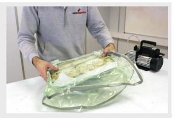
...making it possible to cure multiple parts at the same time in a small oven.
