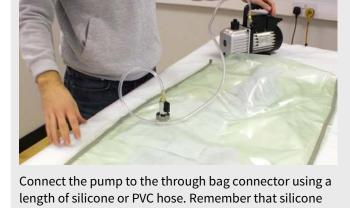
hose must be used on the part is in the oven.
