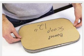
A soft material like Coremat is excellent for making templates for very contoured shapes.
