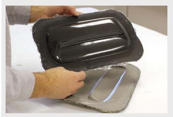
This bonnet scoop has a high gloss finish straight out of the mould.
