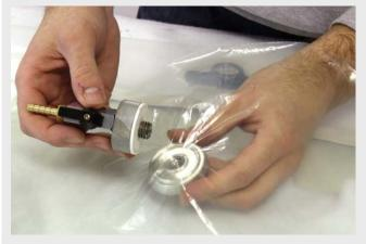
Pass the threaded part of the connector through the hole in the film and place the other half inside the bag.
