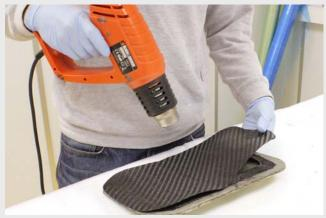
Remove the protective film from *both sides* of the Vari-Preg 400g backing ply.
