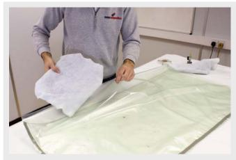
Load the part(s) into the envelope bag, facing upwards.
