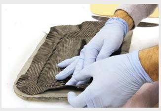
Continue to work the prepreg, gently smoothing and shaping it into the contours of the mould.
