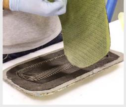
Backing film is removed from prepreg carbon fibre before laminating.
