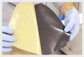
Carefully peel the backing paper away from the Easy-Preg surfacing ply. Only one side has a resin film.
