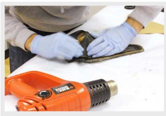
A very contoured shape like this NACA duct requires gentle application of heat to make the prepreg more pliable.
