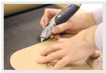
Instead of cutting, a Stanley knife blade is used at a right angle to 'score' the Easy-Preg to mark it.
