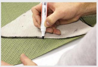
The backing ply can easily be marked using a permanent marker pen on the removable film.
