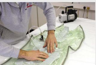
Push and pull the bag from side to side to free up more 'slack'. The whole surface should have an excess of bag.
