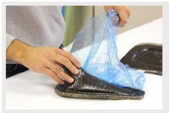
Release film virtually falls off the parts in seconds.
