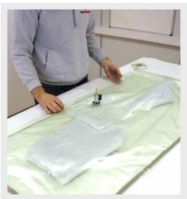
Position the connector in a gap in the bag, on some breather connected to the part(s).
