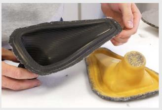
This NACA duct has a satin finish because the mould itself is satin finished.
