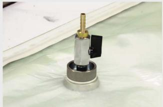
Screw the two halves together tightly to complete the through-bag connector fitment.
