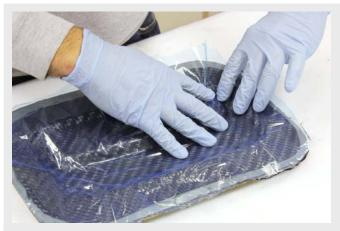
The film should comfortably cover the whole part. Don't worry if it's oversized or wrinkled but ensure the film is not 'tight' and does not 'bridge' anywhere on the part.
