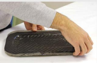
Releasing parts is simply a matter of sliding a fingernail or plastic card under an edge of the cured laminate.
