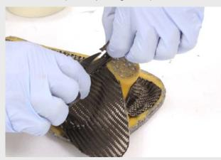
Composites Snips are useful for snipping off small excesses of material
