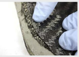
Having cut the backing ply smaller than the surface ply, a small amount of surface layer should extend past the backing layer all the way around the mould.
