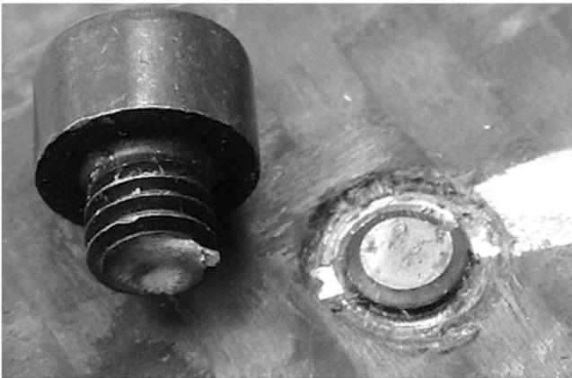
Fig. 17. Bolt failure in torsion tests.
